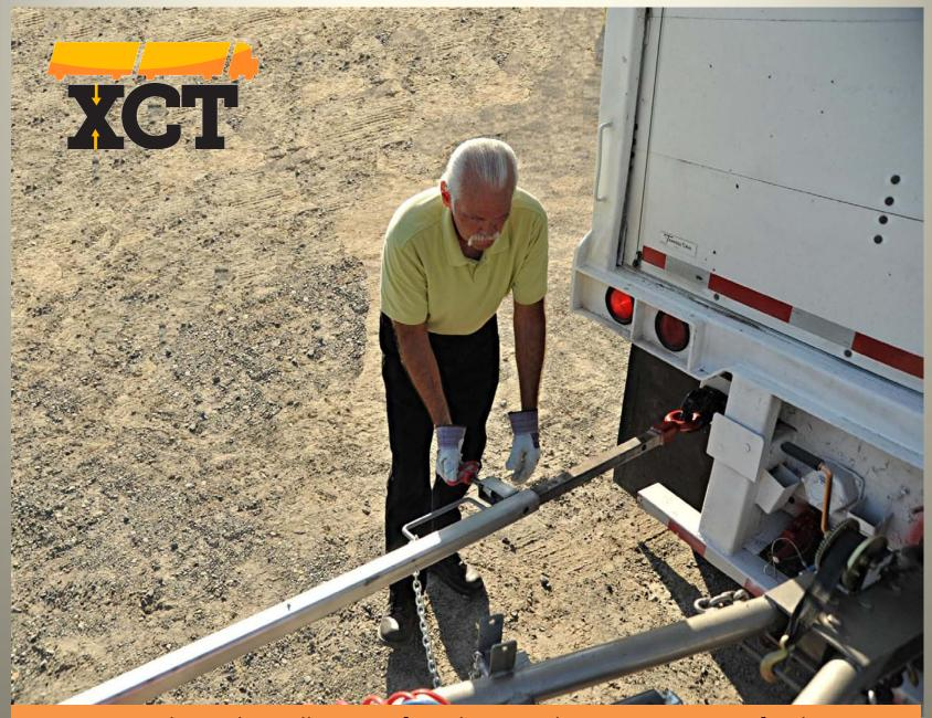
Spin the Red Handle Pin to free the inner bar so it can move freely.
