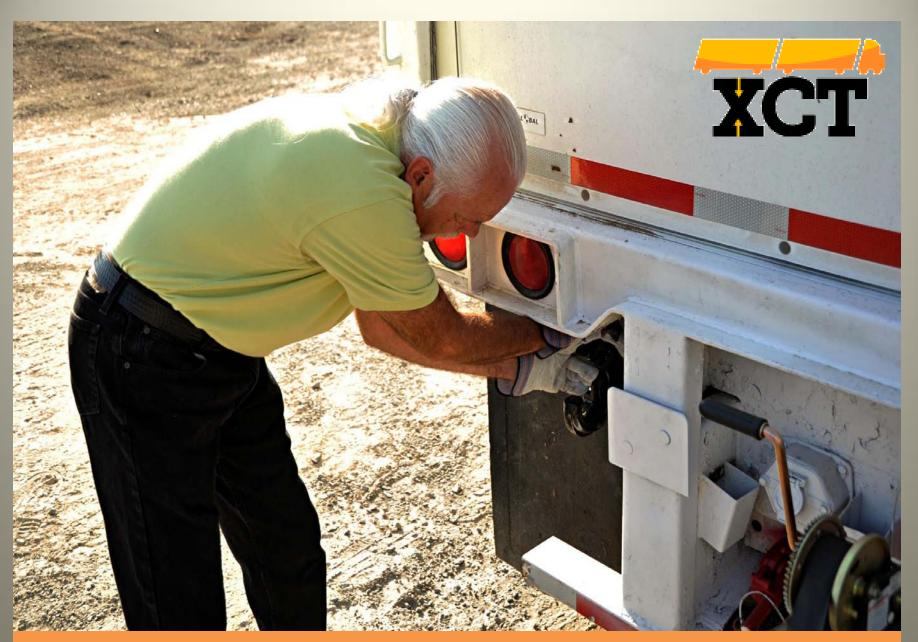
Exit the cab and start the XCT connection process by ensuring the 15 ton pintle hook is open and ready for use.
