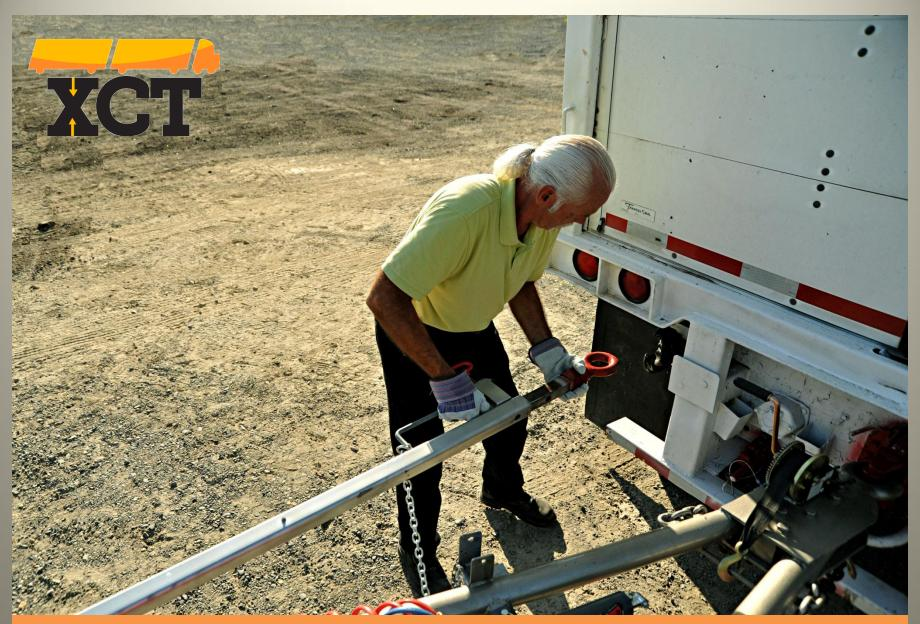
Pick up the XCT from the dolly, with your left hand behind the eye bolt, and connect the XCT to the pintle hook.
