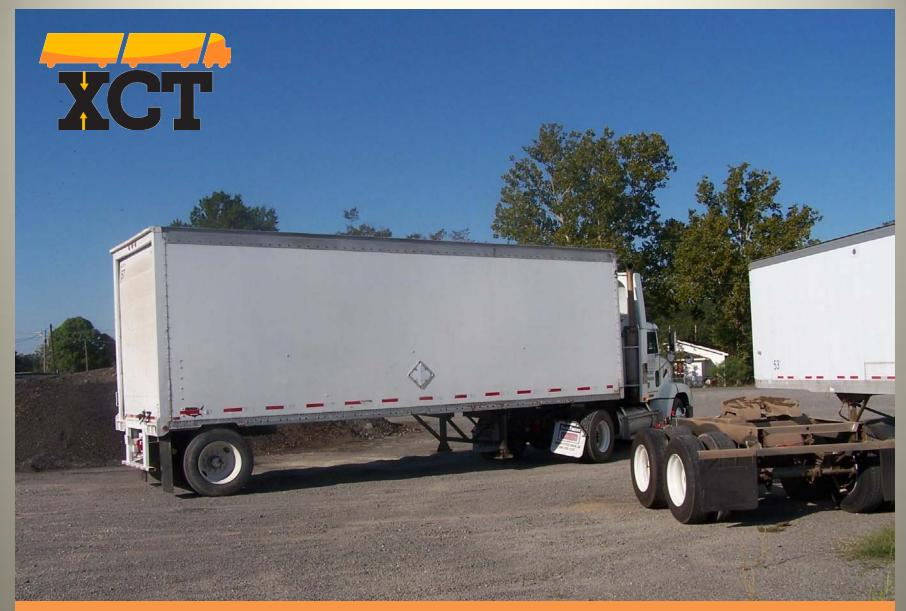
Pull to the front of the dolly. There is no need to stage the dolly when using the XCT.
