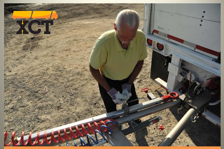
Remove the latch pin which secures the XCT to the dolly.
